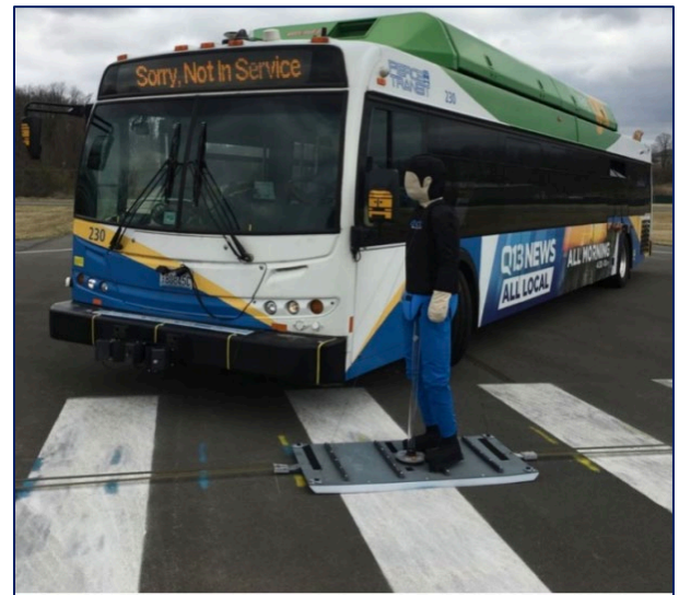
Figure 2: A bus stopping for a VRU mannequin (Source: Virginia Tech Transportation Institute).
